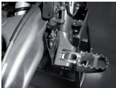
Footrest bracket and springs
