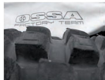
Tyre in bad working condition
