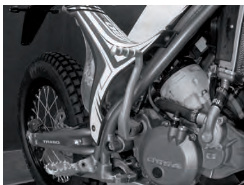
Engine kick-start pedal joints
